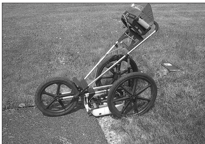
Figure 2. GPR Roots Inspection System. The SIR-3000 Control Computer is at the top with its sun shield. The radar antenna is the module in the white tub (which maintains contact with the ground surface). An encoder wheel rubs against the cart's right rear wheel to provide distance information for automatic data collection.
